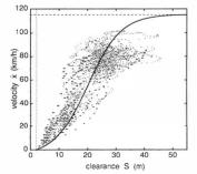
The model has a few drawbacks since the acceleration does not depend on the speed difference. That is, it does not matter if the leader is faster or slower than the following vehicle.
