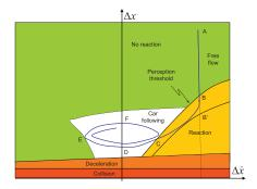
The x-axis represents the speed differential and the y-axis is the spacing.
