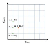
The cumulative counts determine the flow into or out of the link in each time interval, i.e.,  $y(t) = N(t, x) - N(t + \Delta t, x)$  as shown.
