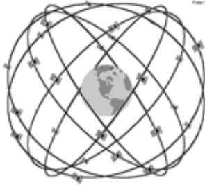
GPS Nominal Constellation 24 Satellites in 6 Orbital Planes 4 Satellites in each Plane 20,200 km Altitudes, 55 Degree Inclination
