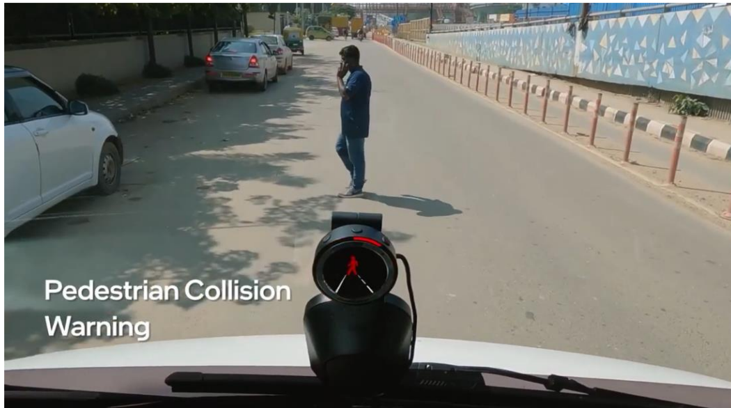
Figure 15: Demonstration of pedestrian collision warning in ADAS-equipped vehicle
