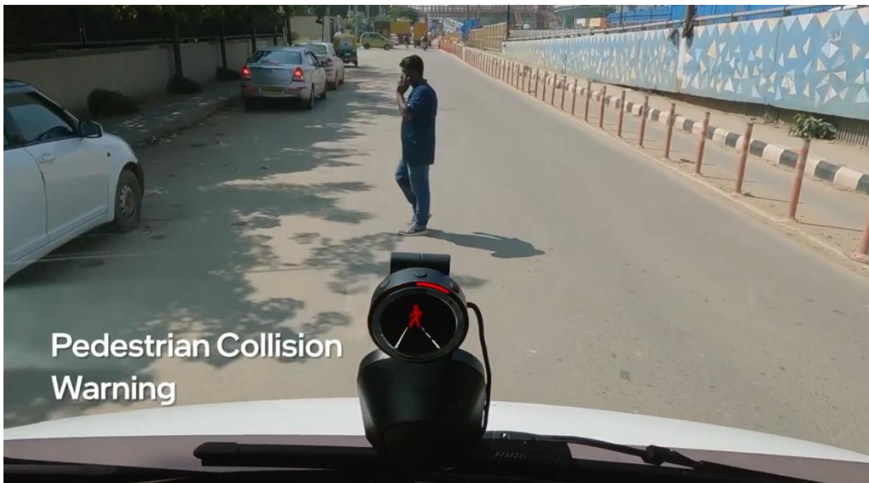
Picture 11: Demonstration of pedestrian collision warning in ADAS equipped vehicle
