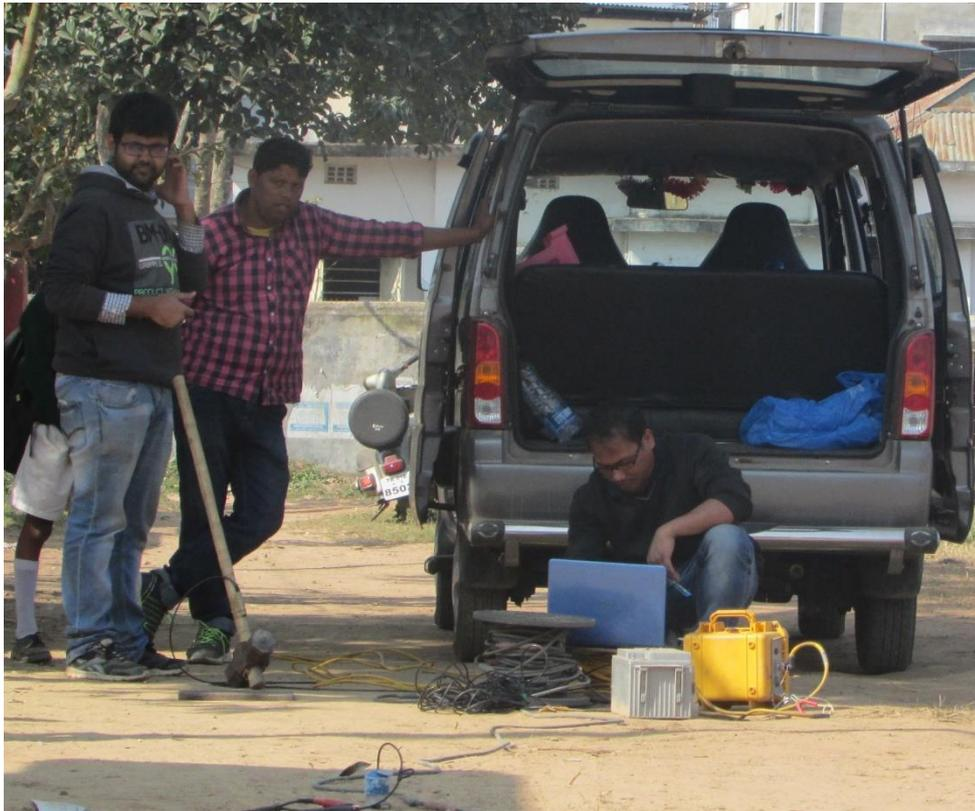
Figure 3. Multichannel Analysis of Surface Wave (MASW) test at one of the damaged locations in Tripura
