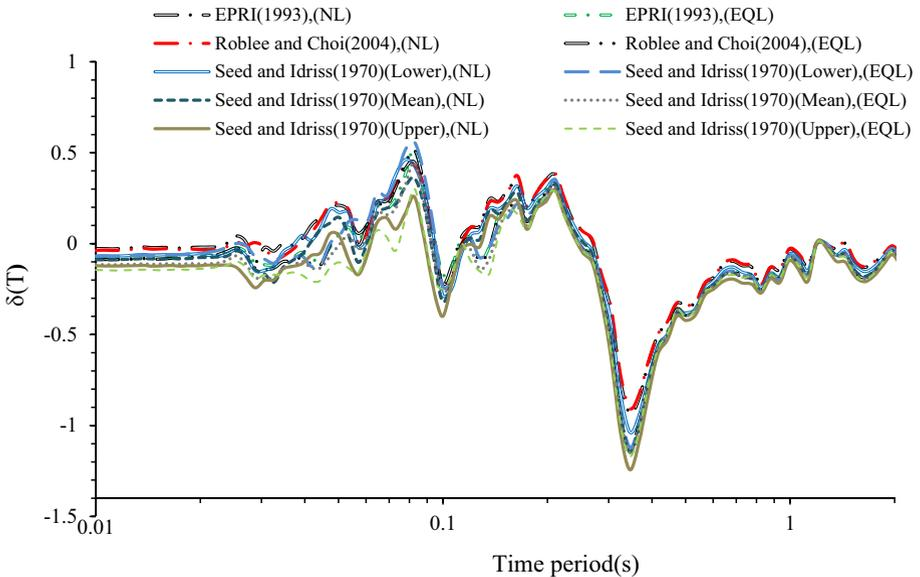
**Fig. 12** Variation in residual with time period for different modulus reduction and damping curves at sand site FKSH08
