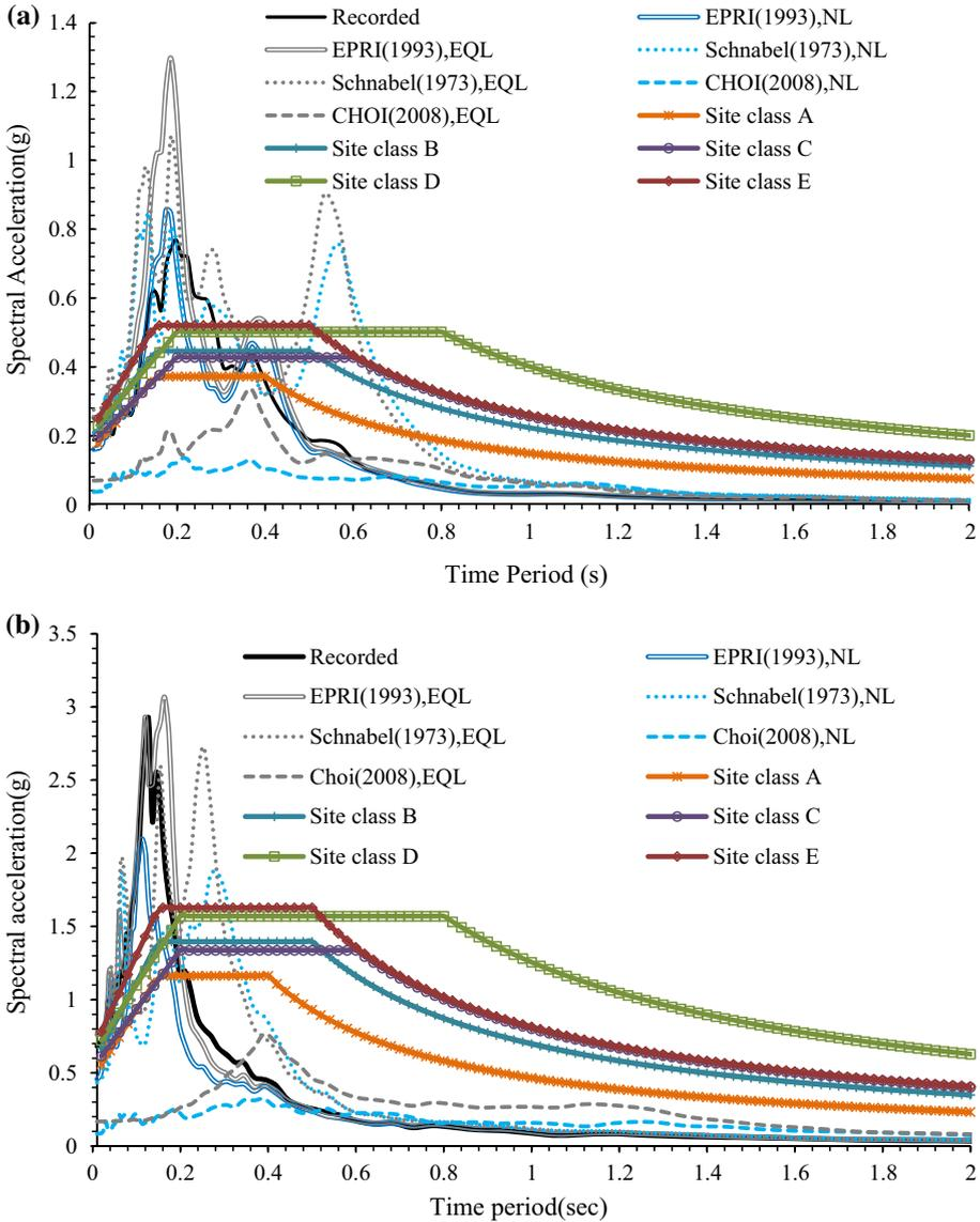
**Fig. 3** Variation in response spectra for different modulus reduction and damping curves at **a** LP rock site FKSH18 **b** LG rock site IWTH27
