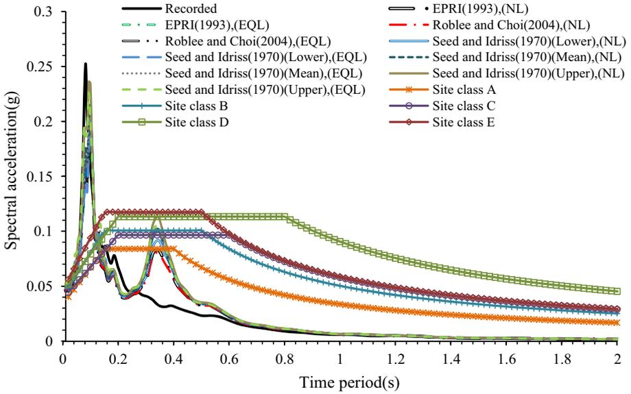
**Fig. 11** Variation in response spectra for different modulus reduction and damping curves at sand site FKSH08
