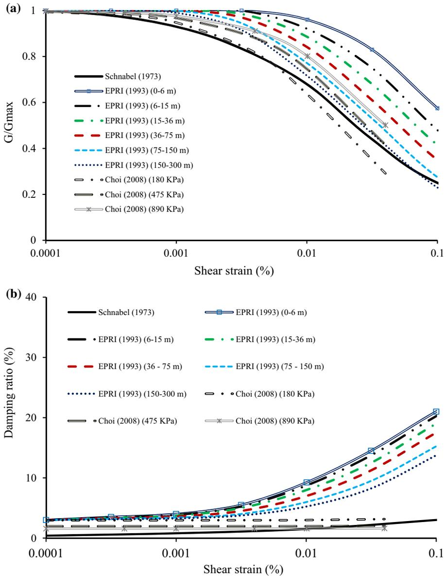
**Fig. 2** Variation of shear modulus (a) and damping (b) with shear strain for rock
