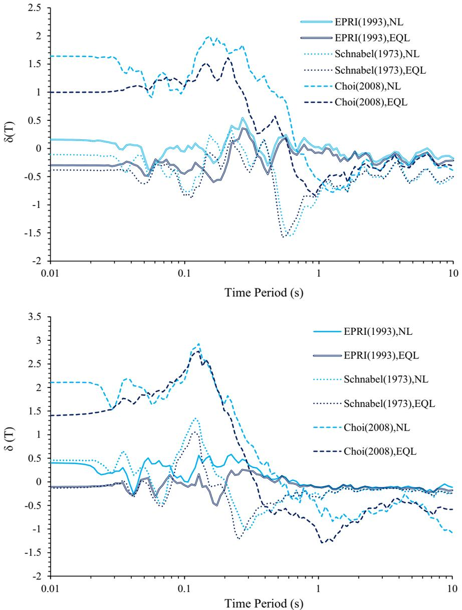
**Fig. 4** Variation in the spectral residual with time period for different modulus reduction and damping curves **a** LP rock site FKSH18 **b** LG rock site IWTH27
