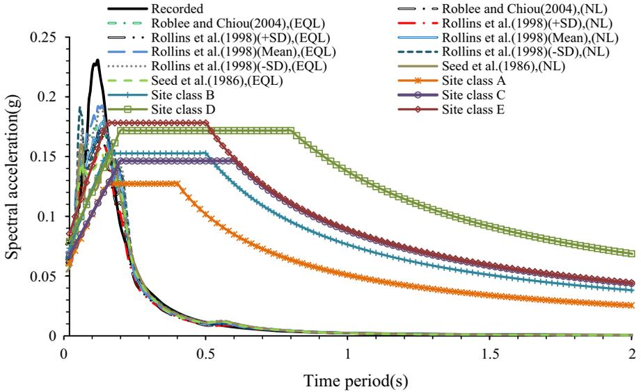
**Fig. 7** Variation in response spectra for different modulus reduction and damping curves at LG gravel site TKCH08
