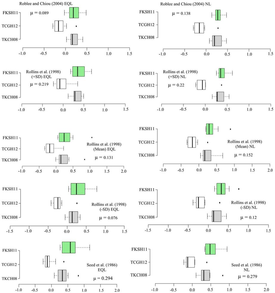
**Fig. 9** Variation of the bias in the residual of the response spectra for gravel profiles considered in the analyses
