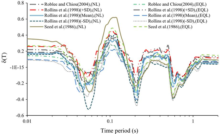
**Fig. 8** Variation in residual with time period for different modulus reduction and damping curves at LG gravel site TKCH08
