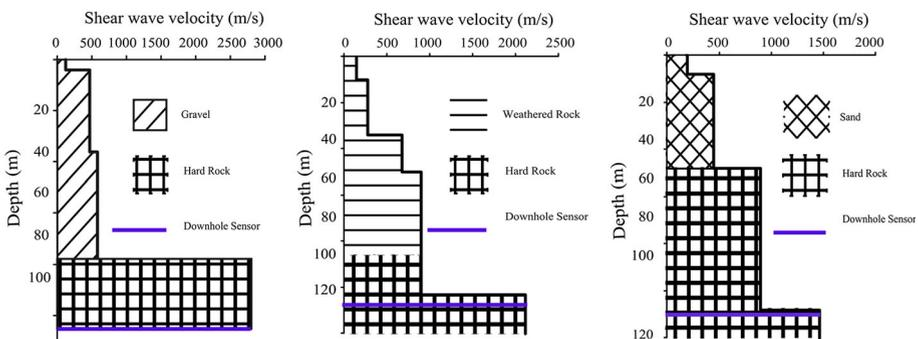
**Fig. 1** Typical shear wave velocities of soil columns of rock (IWTH08), gravel (TKCH08) and sand (FKSH08), from the KiK-Net database
