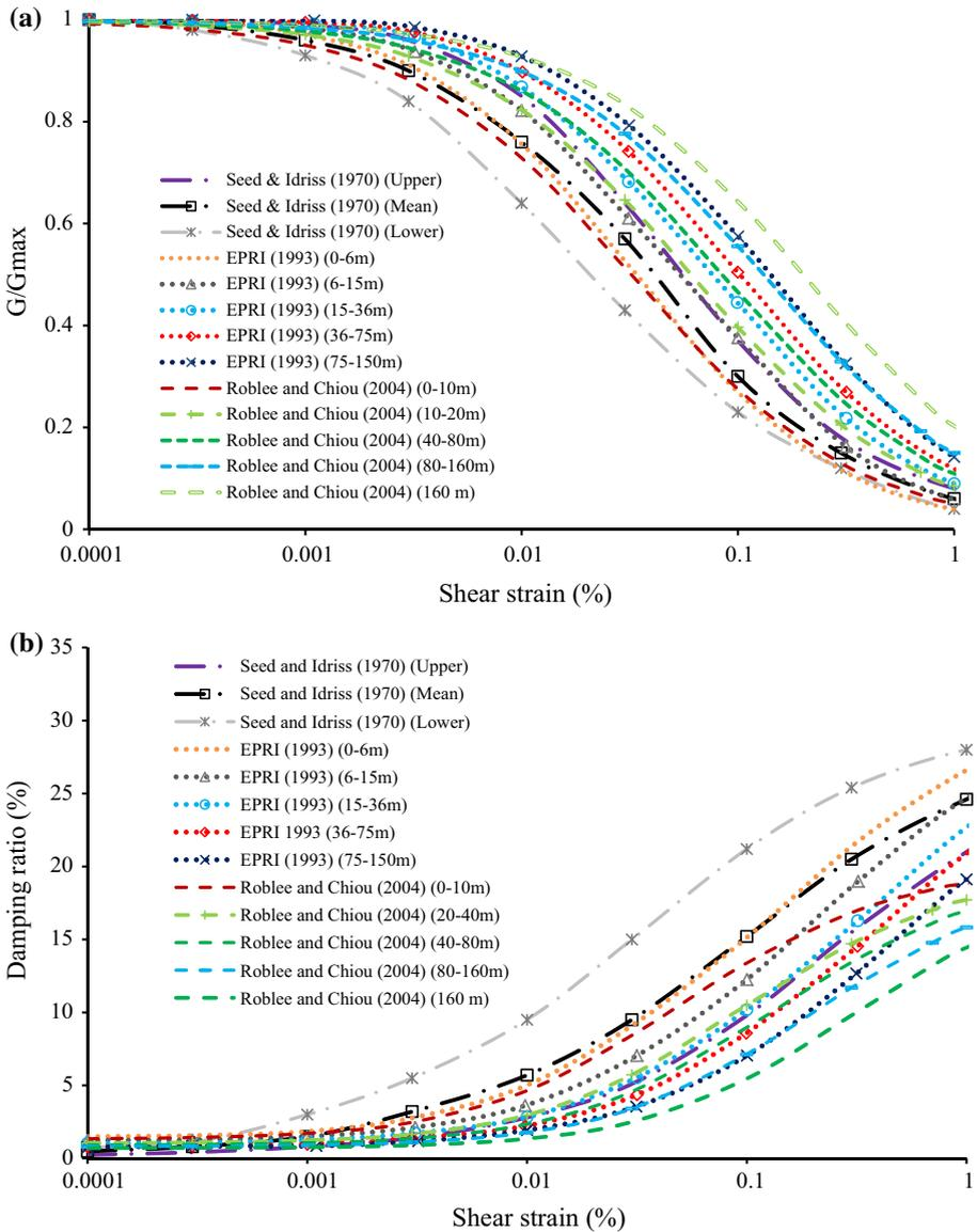
**Fig. 10** Variation of shear modulus (a) and damping (b) with shear strain for sand
