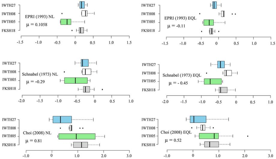
**Fig. 5** Variation of the bias in the residual of the response spectra for rock profiles considered in the analyses
