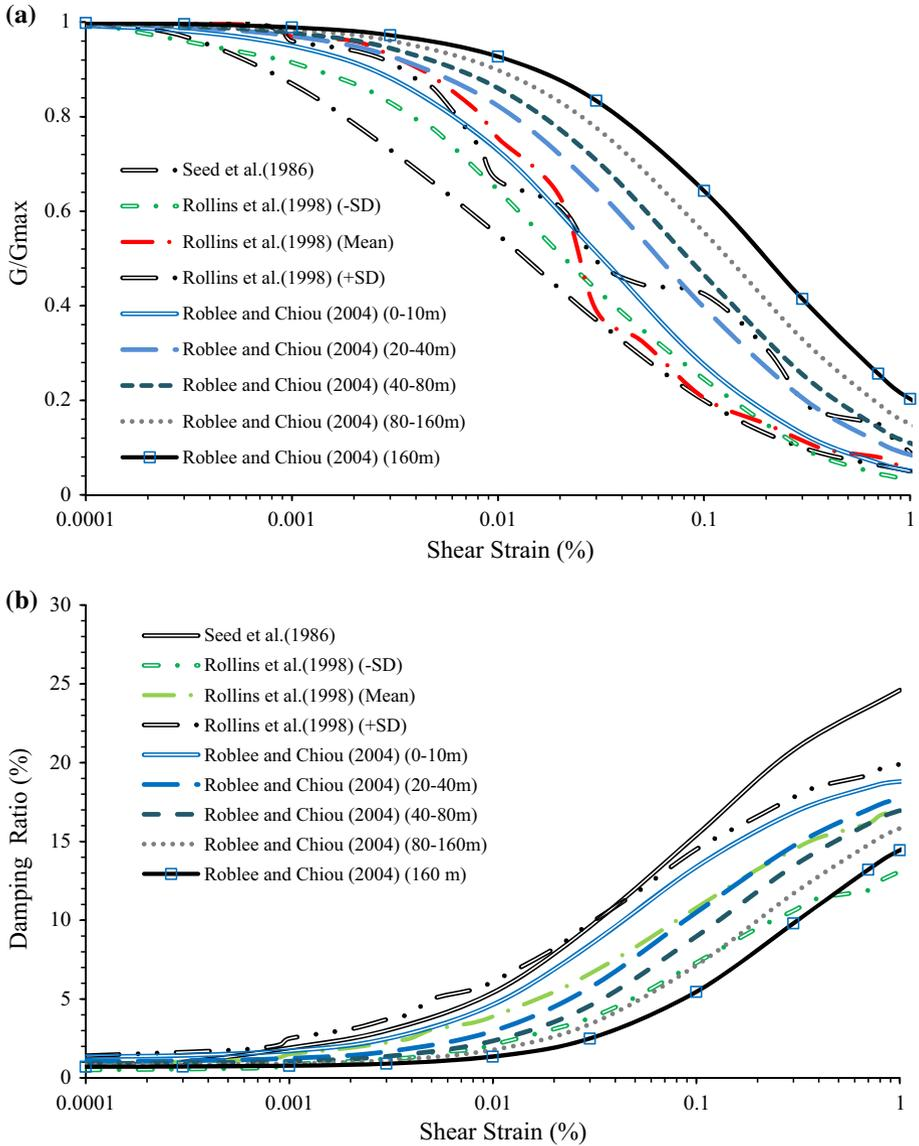
**Fig. 6** Variation of shear modulus (a) and damping (b) with shear strain for gravel
