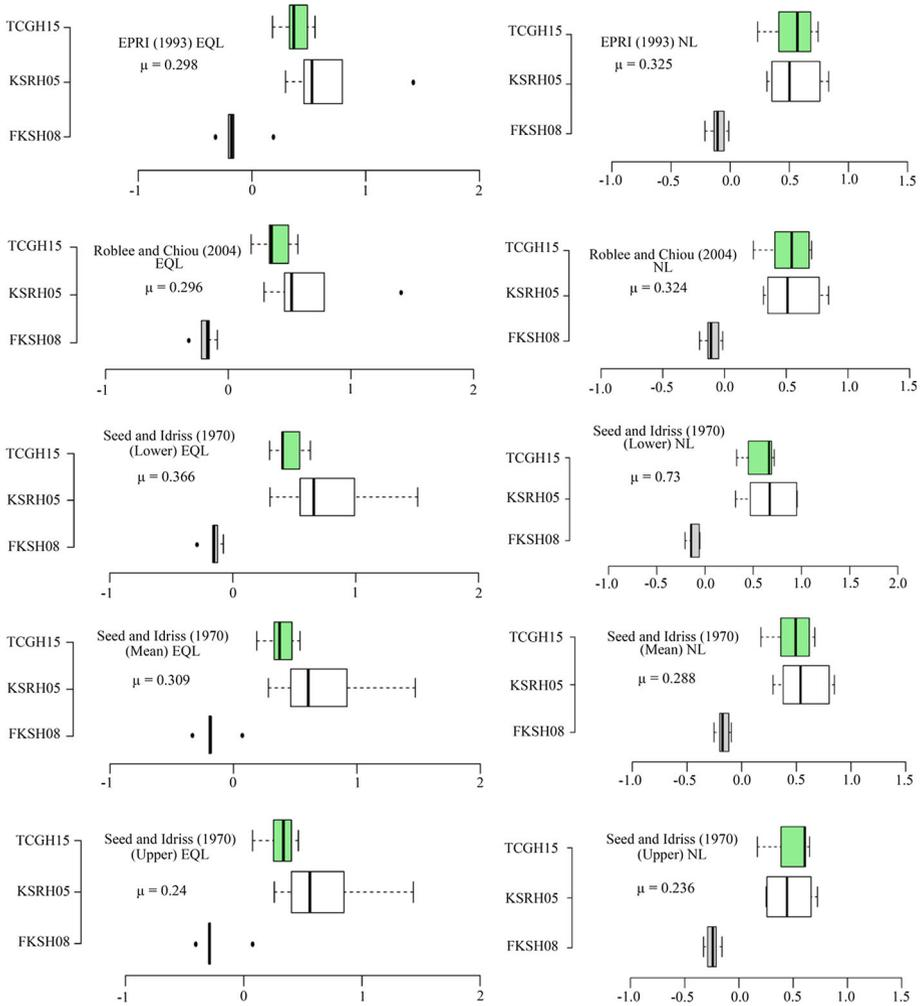
**Fig. 13** Variation of the bias in the residual of the response spectra for sand profiles considered in the analyses
