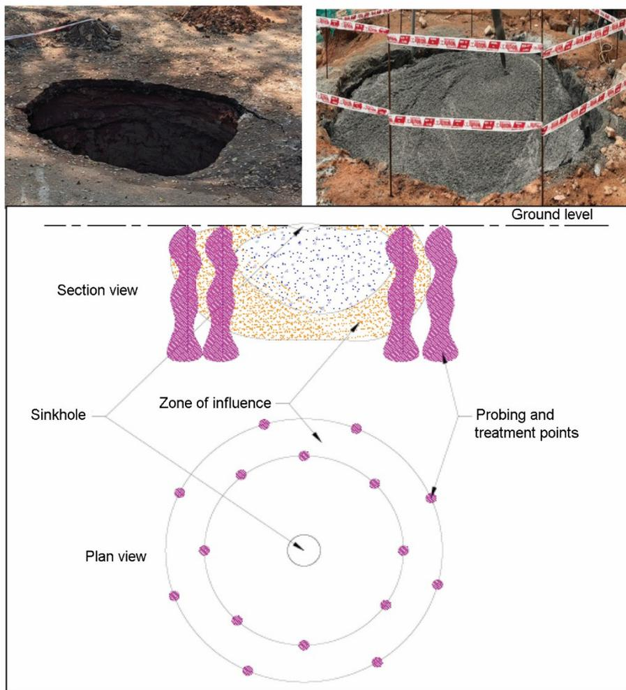
**Figure 9.** Treatment of urban cavity close to a metro project.
