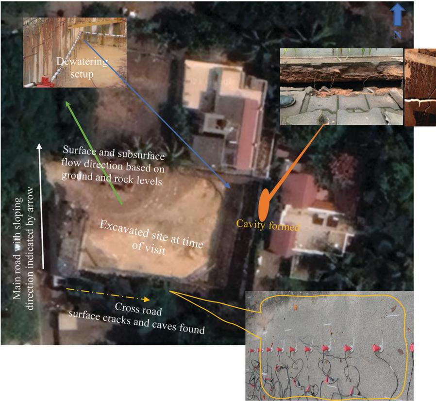
Figure 4. Typical surface cracks and cavity formation due to excavation and dewatering.
