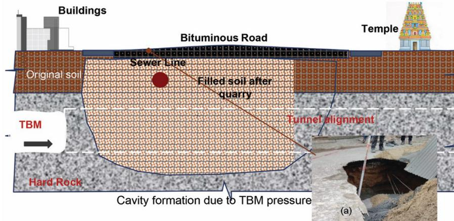
Figure 6. Blow-out cavity formation due to underground tunnelling work in a city.
