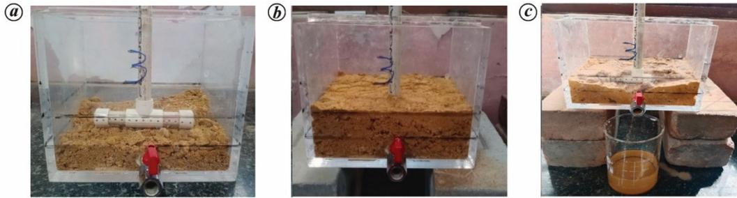
**Figure 8.** Typical experiment to simulate water leakage from a pipe. *a*, Mould filled with soil and underwater pipe. *b*, Soil filled with leakage from pipe. *c*, Soil layer after pipe leakage and the soil fines are lost.
