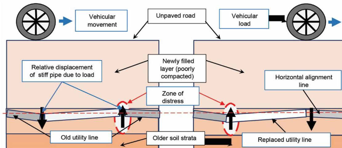
**Figure 7.** Breakage of utility pipes (laid in poorly compacted backfill) due to uneven settlement of surrounding media caused by uneven compaction from vehicular load.
