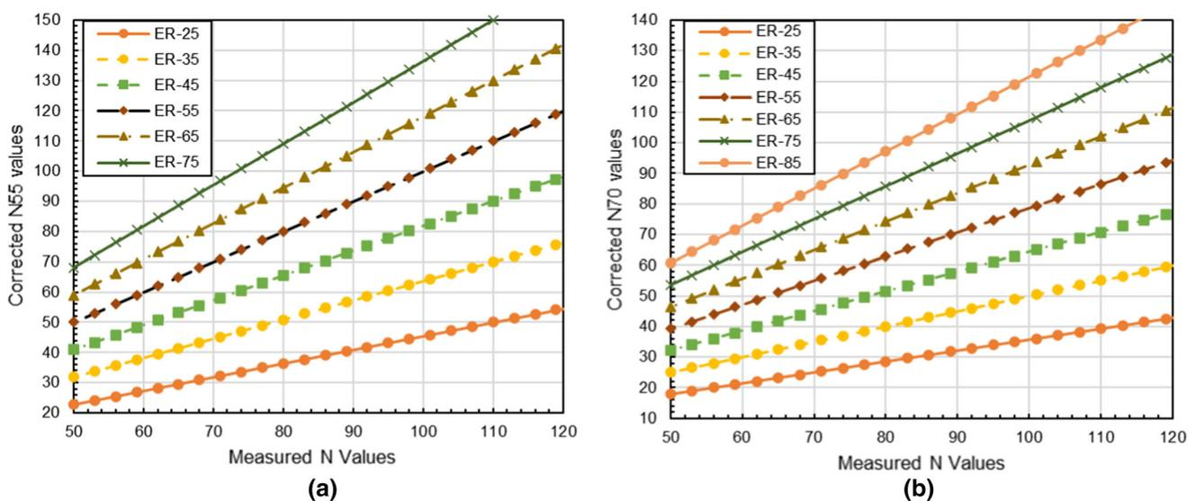
Fig. 2 Rebound *N*-values measured for different energy and corrected *N*-values for reference energy of a 55% and b 70%
