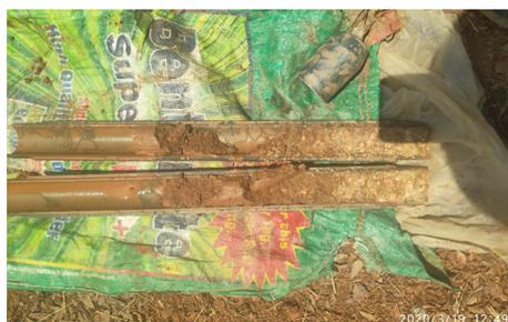
**Fig. 12** Recovered intact medium to dense soil sample beyond rebound layer
