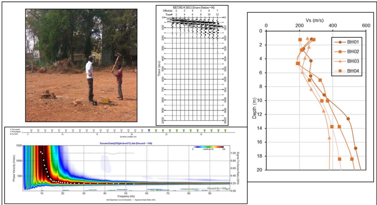
**Fig. 15** Plot of shear wave velocity profiles from MASW of all the four boreholes
