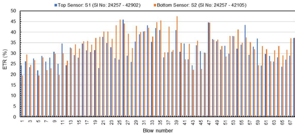
**Fig. 8** Typical plot of ETR variation of top and bottom sensor for each hammer blow at a given depth
