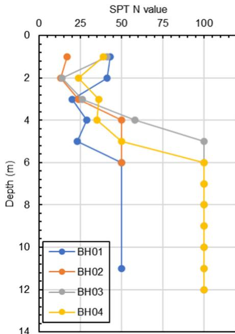
Fig. 5 Plot of recorded N-value versus borehole depth
