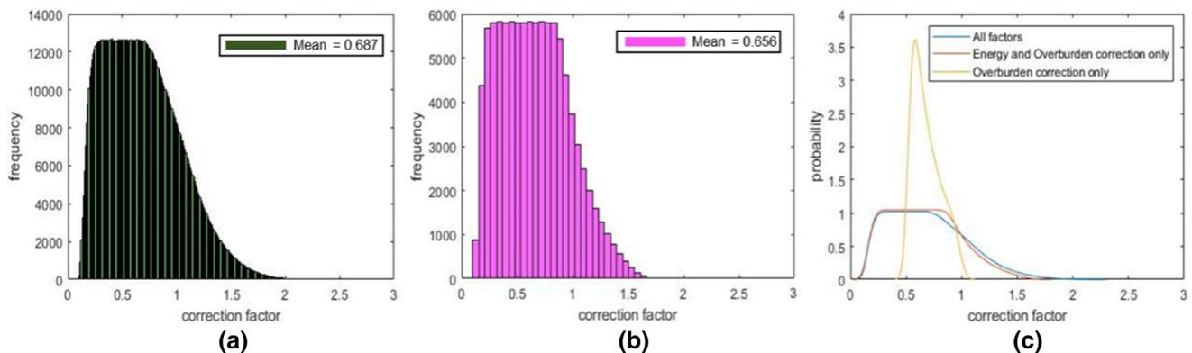
**Fig. 1** Histogram of the frequency of the correction factors obtained after the analysis for considering **a** all five corrections and **b** only energy and overburden corrections, respectively, **c** shows the probability density comparison of the two cases
