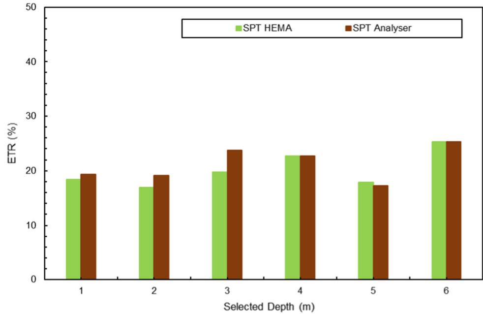
**Fig. 10** The energy transfer ratio (ETR) variation in the top sensor of all four boreholes for each *N*-value measurement
