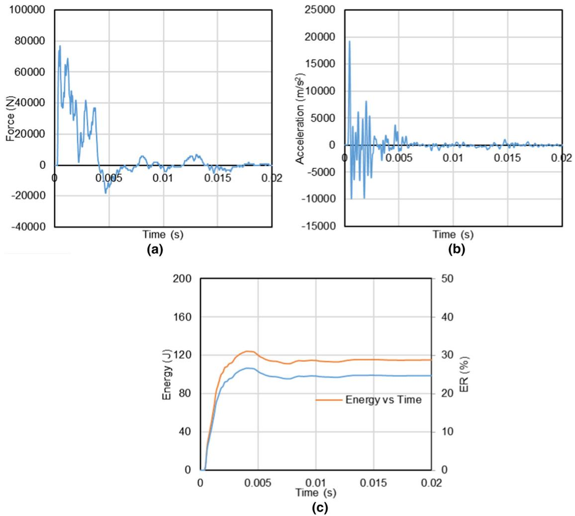
**Fig. 7** Typical **a** force and **b** acceleration variation with time and **c** energy estimated as per ASTM D4633 (2016) from the site
