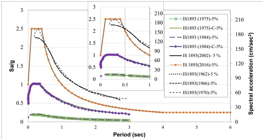
**Fig. 1.4** Average acceleration spectrum curves and response spectra at rock site presented in IS 1893 from 1962 to 2016
