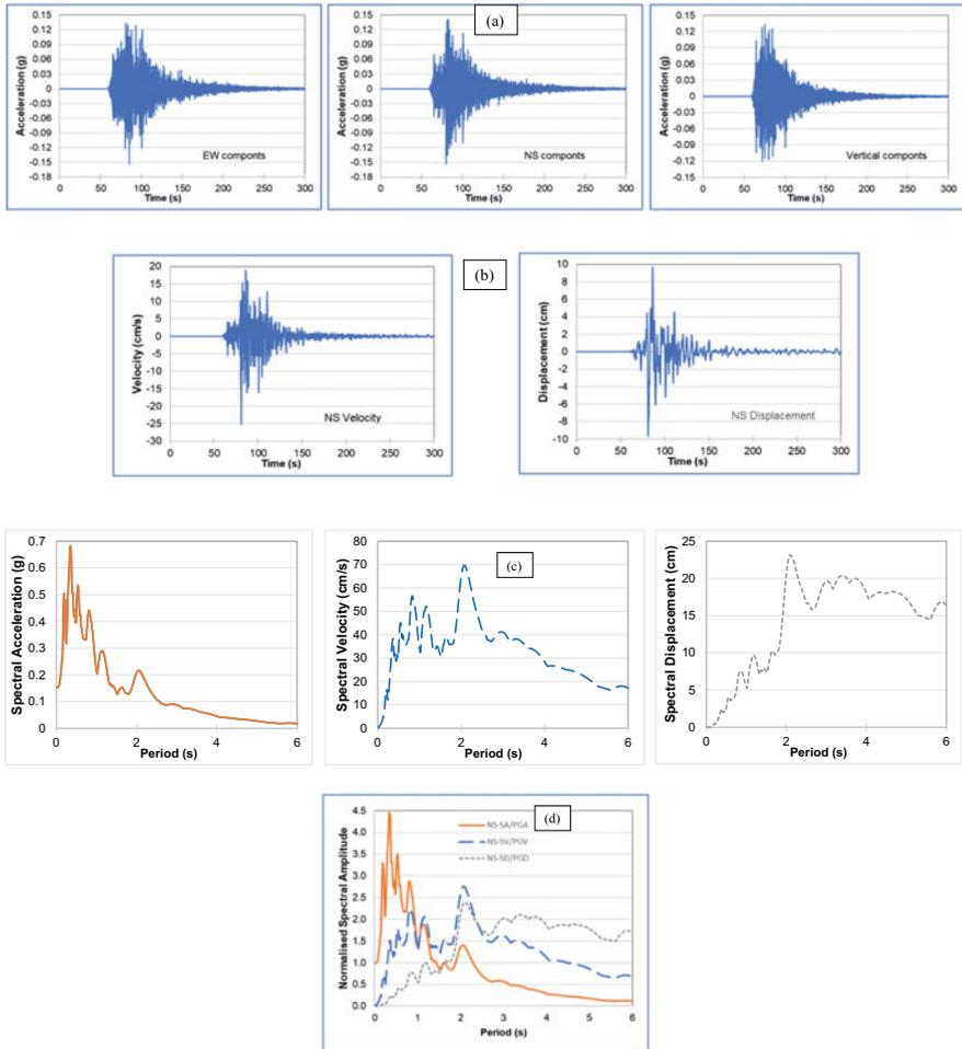
**Fig. 1.5** Typical rock site earthquake time history and response spectrum **a** Acceleration time history of EW, NS, and Vertical record, **b** Maximum (NS) Velocity and Displacement time history data, **c** Response spectrum for acceleration, velocity, and displacement data and **d** Normalised spectral amplitude of acceleration, velocity, and displacement with respective peak values
