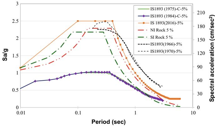
**Fig. 1.14** Newly developed horizontal spectrum using Indian data and 5% acceleration, velocity, and displacement spectrum at rock sites for North India (NI) and South (SI) and also comparison with different versions of IS 1893 spectrum. IS 1893 [6, 7] spectrum with secondary Y-axis
