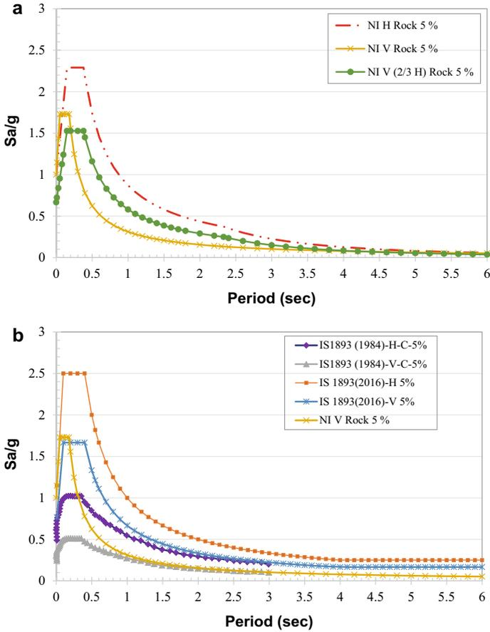
**Fig. 1.15** Comparison of **a** proposed vertical (PV) design response spectrum with horizontal design spectrum and 2/3 factor of horizontal spectrum values for bedrock condition with 5% damping for in NI. **b** Proposed vertical design response spectrum (V) compared with horizontal (H) and vertical (V) suggested in IS:1893 [11] and (1985)
