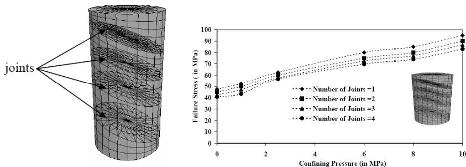
**Figure 35: FLAC 3D Simulation of jointed rock sample of Agra Sandstone subjected to triaxial compression**
