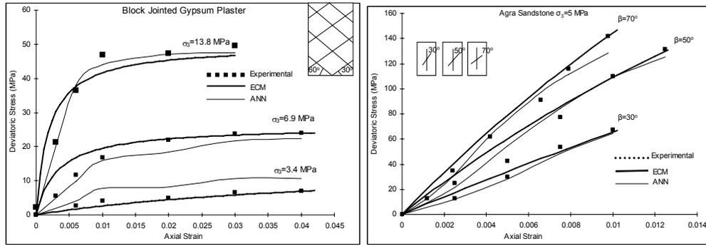
**Figure 39: Comparison of stress-strain curves predicted by ECM and ANN with experimental measurements for jointed rocks**
