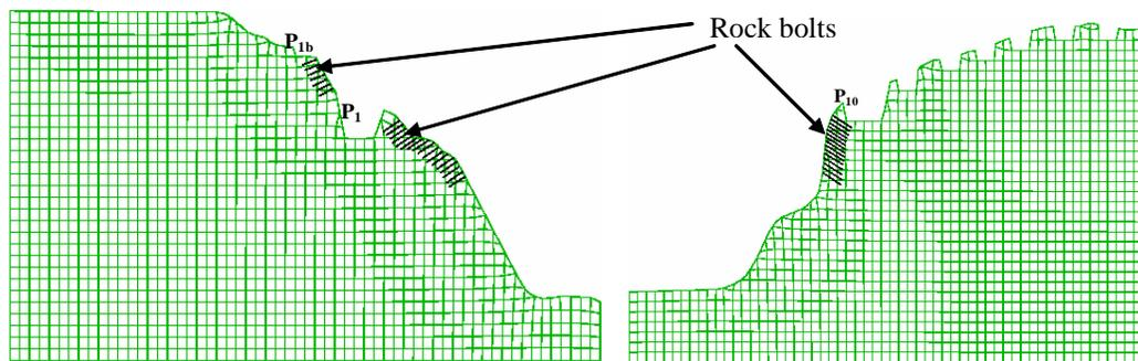
**Figure 38: Rock bolting scheme proposed for Anjikhad slopes**
