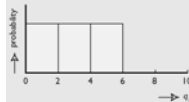
Histogram showing an equal 1/3 probability that the values of the random variable Q_t will be in any one of the three two-flow unit intervals.
